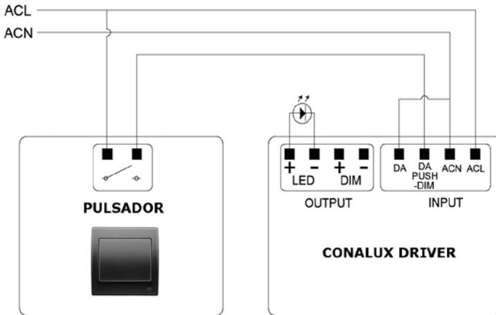
ESQUEMA CONEXIÓN PUSH MÚLTIPLE CONALUX 12-40W (SIN CABLE SYNC):
